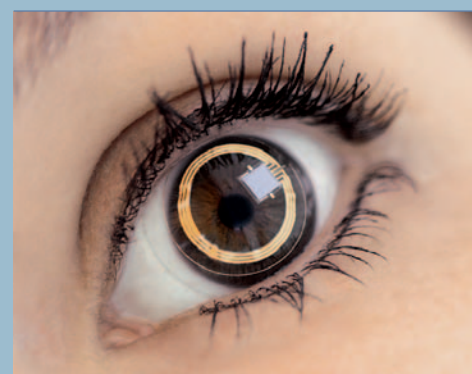
SENSIMED Triggerfish ® Sensor in the eye
